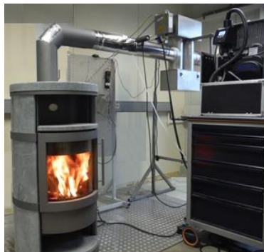
Fig. 9. ESP-S precipitator downstream the stove
