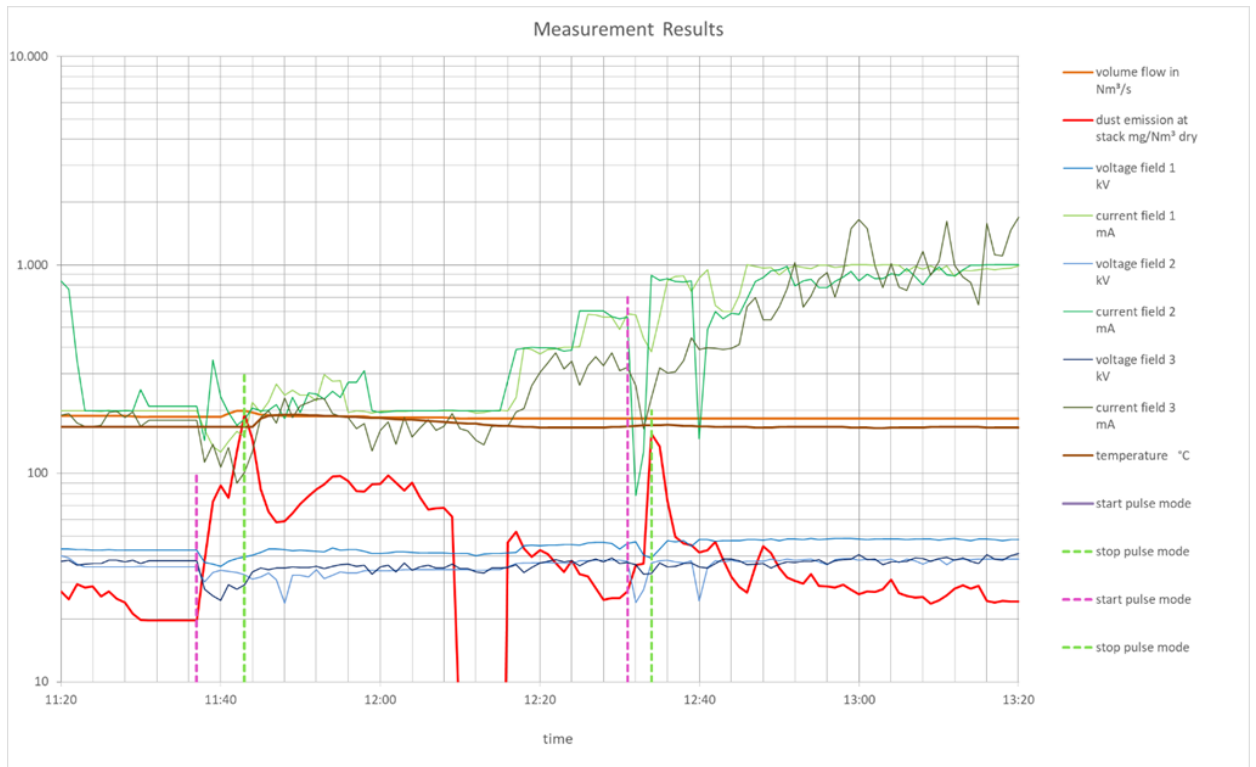
Fig. 7: Clean gas dust content (red line) with smooth DC from a 3-phase TR set. Interruptions through short pulse mode operation times at about 11:40 h and again at 12:35 h.
