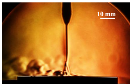
Fig. 13 Schlieren image of streamer corona. (14 kV, 18 °C, 45%, 1013 hPa)
