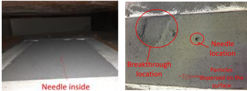
Figure 4 Dust explosion after breakdown in the vicinity of the needle
